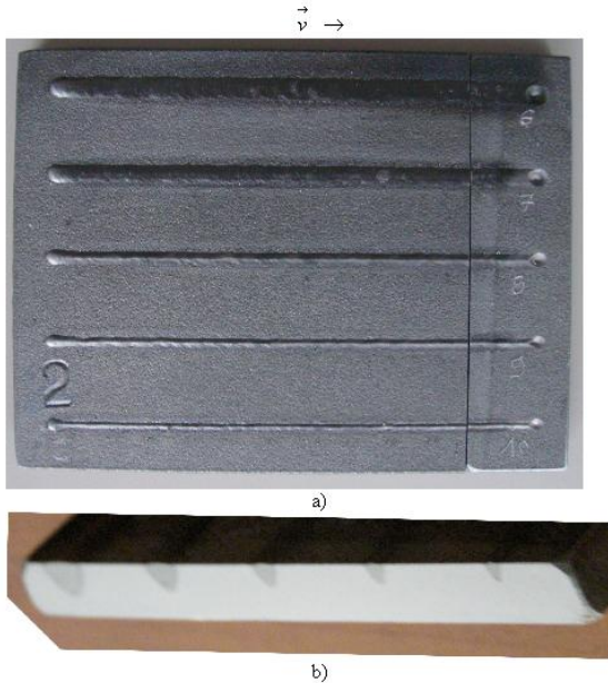
Fig.1 Steel plate with welds a) Plate surface b) Cross section through plate
